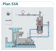
Circulation with External Buffer Fluid Tank
