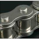
Chain "stretch" is a result of wear on the pin and bushing, requiring costly chain adjustments or replacement. Conventional lubricants do not penetrate tight tolerances and, therefore, provide minimum benefit. Chesterton's chain lubricants are formulated
